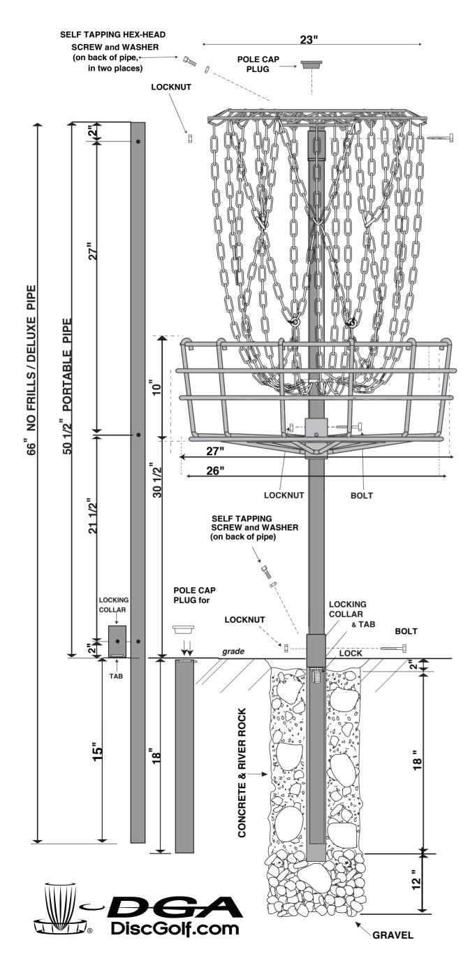
POLE (66 in.) - 1 1/2 in. I.D., 1 15/16 in. O.D. hot-dipped galvanized pipe, drilled.
